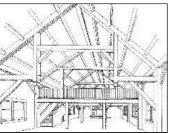
The log cabin marks the beginning of American architecture. The roof typically was timber frame with load bearing exterior log walls. Timber frame is a traditional method of post and beam construction defined by the use of wood to wood joinery. In timber frame construction the structural components remain exposed to the interior. Their geometry functions as an integral decorative element and may be used to achieve most any architectural style.
